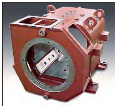
Joliet C75ZB New Drilling Frame Opposite Drive End View
